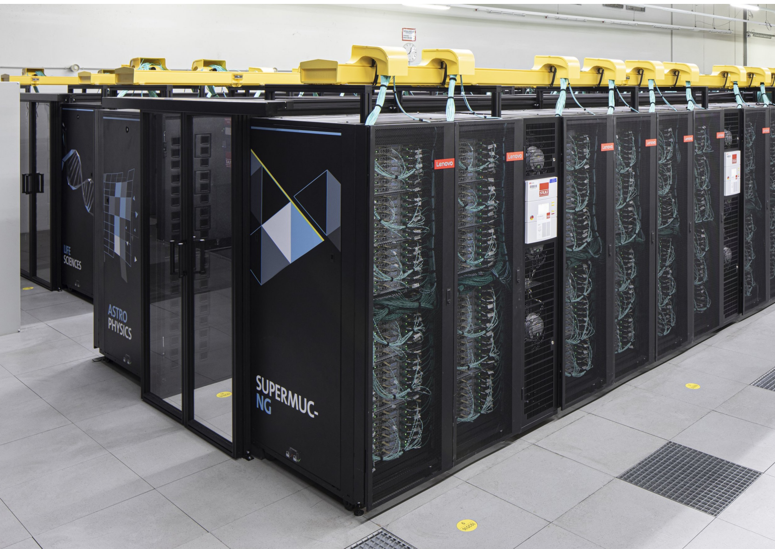
The high-performance computer SuperMUC-NG at the Leibniz Supercomputing Centre is based on Lenovo ThinkSystem SD650 DWC compute nodes and equipped with Intel Skylake Xeon Platinum 8174 processors. The machine hosts 6,336 thin compute nodes, each with 48 cores and 96 GB memory, and 144 fat compute nodes, each with 48 cores and 768 GB memory per node. User operation started in August 2019. (Picture: F. Löchner).
