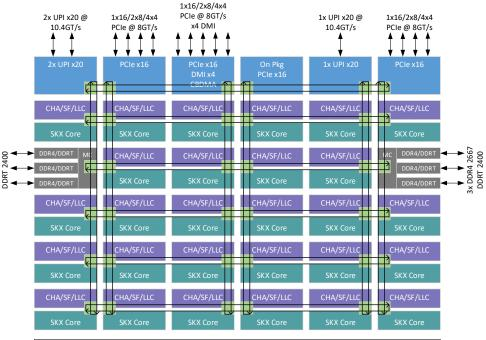
CHA – Caching and Home Agent; SF – Snoop Filter; LLC – Last Level Cache; SKX – Skylake Server; UPI – UltraPath Interconnect Power Management: Per Core P-State (PCPS) Uncore Frequency Scaling (UFS) Energy Efficient Turbo (EET) On die PMAX detection (NEW) Intel® Speed Shift Technology (NEW)
