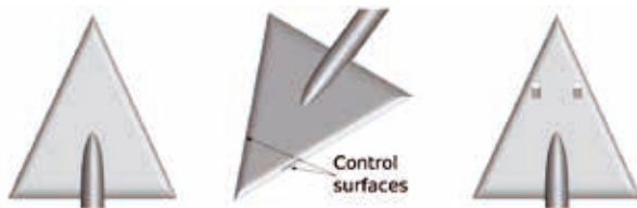
Figure 3: Configuration without flow control (left), with control surfaces in the front part of the wing (center), and with slots in the front part of the wing (right) [5].
