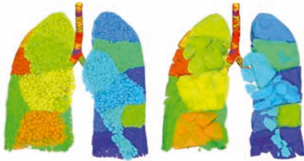
Figure 3: Algebraic multigrid aggregates for the fine level (left) and the coarse level (right) representation of the human lung model.
