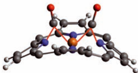
Figure 1: DFT model of dicarbonyl bonding at saddle-shaped cobalt tetraphenyl-porphyrins anchored on well-defined coinage metal substrates like Cu and Ag. The Ag(111) surface considered here and the phenyl substituents have been removed for clarity.
