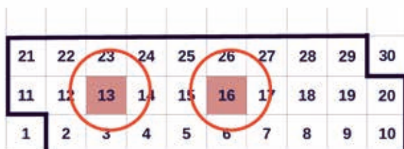
Figure 1. Hyperthreaded sliding window (represented here in two dimensions, instead of three as in the actual code), employed by the ls1 mardyn version optimized for the Intel Sandy Bridge EP architecture. At the present stage, the two highlighted cells 13 and 16 are concurrently processed by SMT threads. Thereby, cell 2 is considered as a neighbour cell for the last time, leaving the sliding window, and cell 27 enters the sliding window; cells 28 and 29 are prefetched.
