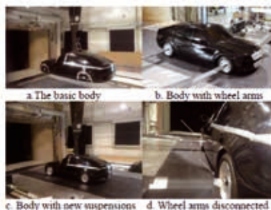
Figure 1: Four different Setups in wind tunnel
