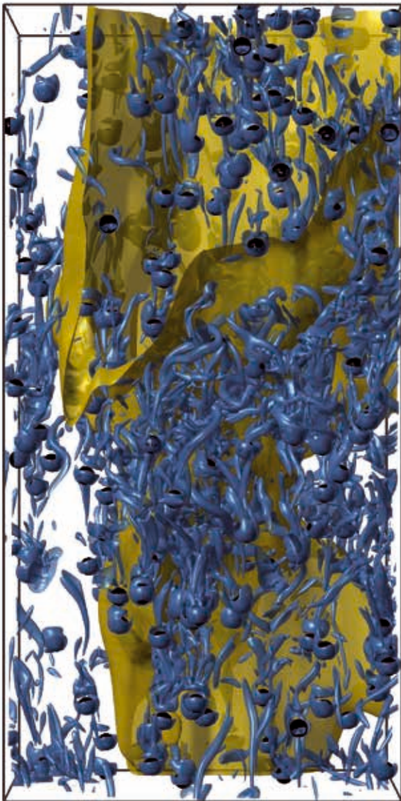
Figure 1: Flow visualization of a sub-volume of the domain (one fourth of each linear dimension is shown): Particles are represented in black, blue surfaces correspond to isosurfaces of the Q criterion and display the wakes of the particles. Isosurfaces of the vertical component of the velocity field are shown in yellow. For the velocity field, the flow has been box-filtered with a box width of approximately 5 particle diameters in order to extract the large scale structure.
