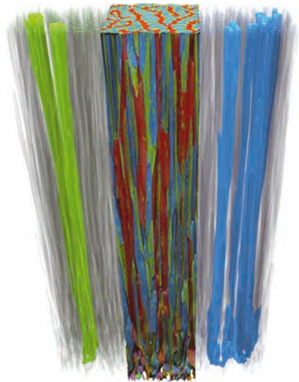
Figure 1: A 800 \times 800 \times 4000 cell simulation of the directional solidified ternary eutectic system Al-Ag-Cu. In green and blue the evolving rods are exempted.
